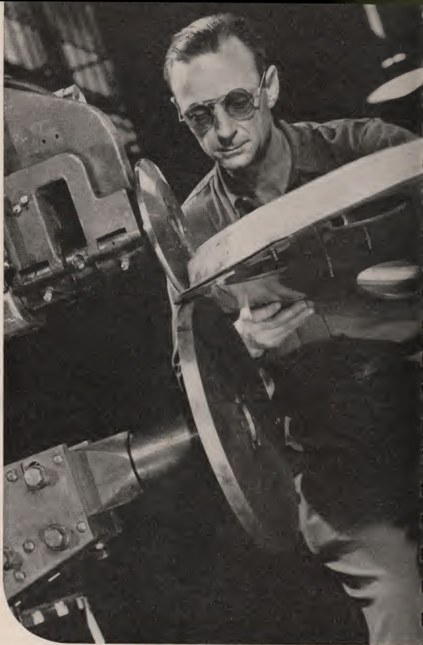
Electric seam welding an aircraft part.
